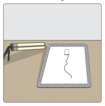
Step 3: Apply adhesive and wall mounting clips
